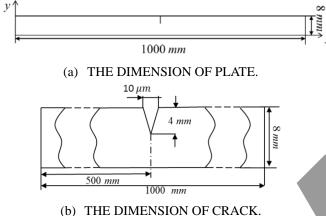
(b) THE DIMENSION OF CRACK. FIGURE 4: THE DIMENSIONS OF A PLATE WITH CRACK.
