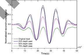
**FIGURE 9:** THE RECONSTRUCTED SIGNALS FOR DIFFERENT RELATIVE DEPTH.
